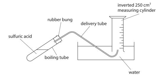
The bung was removed and 0.650 g of copper(II) carbonate was added to 25.0 cm<sup>3</sup> of 2.00 mol dm<sup>-3</sup> sulfuric acid (an excess) in the boiling tube.
